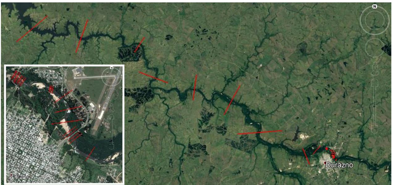
Figure 3–1 Cross-sections of the hydrodynamic model
