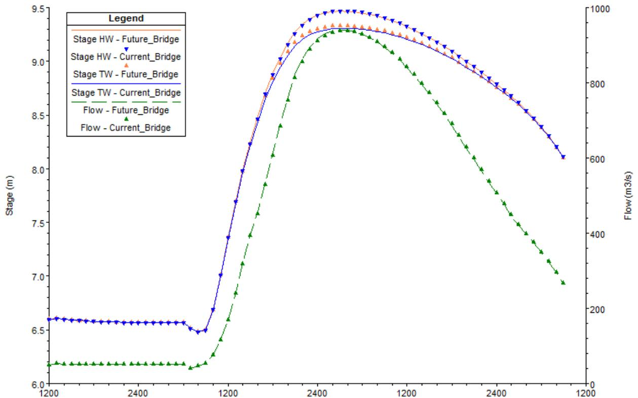
**Figure 3–3 Water levels, referred to the Official Zero, upstream and downstream of the current and future Margat Bridge for Case 1**
