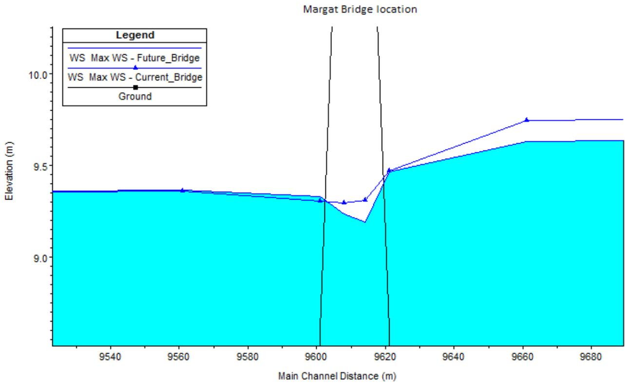
**Figure 3–2 Maximum water level profile focused on the Margat Bridge area with its current and future design for Case 1**
