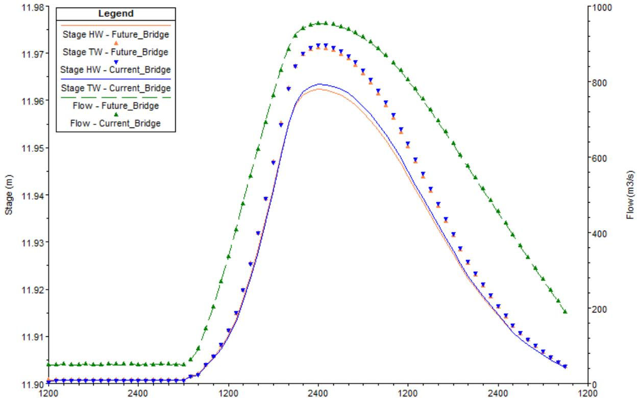
**Figure 3-4 Water levels, referred to the Official Zero, upstream and downstream of the current and future Margat Bridge for Case 2**
