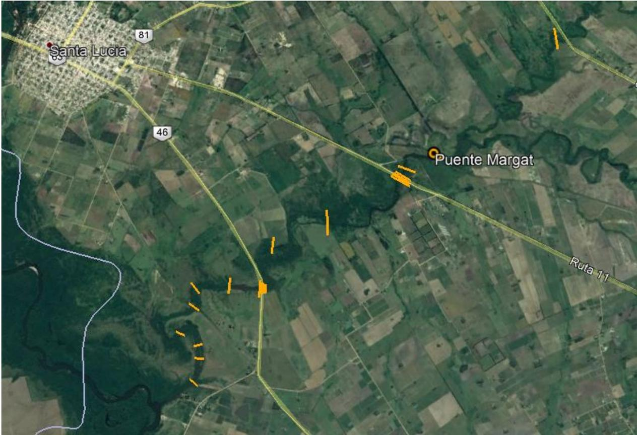
**Figure 3–1 Cross-sections considered for the hydrodynamic model**
